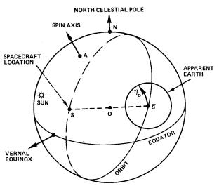
Fig. 1 Celestial coordinate sphere with relative directions.
